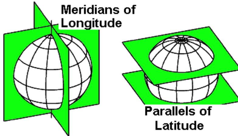
The lines of latitude and longitude form a pattern called the graticule. The lines of constant longitude are called meridians. These all meet at the poles. They are circles of the same radius which is the radius of the earth,  $R_e$ . They are examples of great circles. The lines of constant latitude are called parallels of latitude. They are circles whose radius depends on the latitude. The radius is  $\cos(\phi) R_e$ . Parallels of latitude are examples of small circles.
