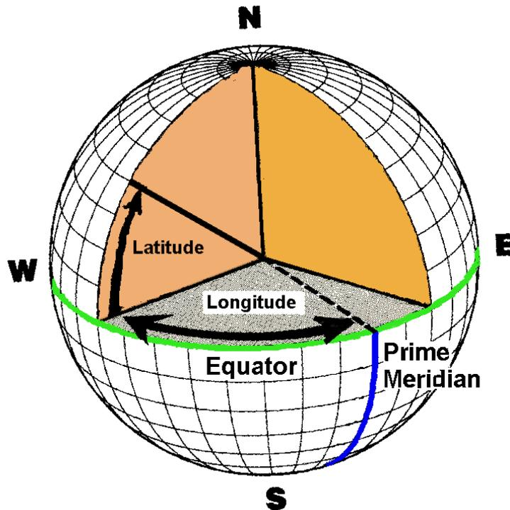
The longitude used in geodesy is positive going east from the prime meridian. The values go from  $0$  to  $360$  degrees. A value in the middle United States is therefore about  $260$  degrees east longitude. This is the same as  $-100$  degrees east.
