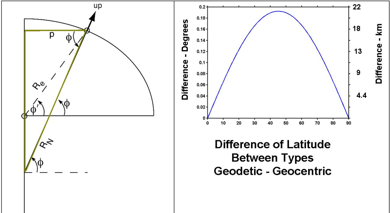
Above on the left is a diagram showing the geodetic ( $\phi$ ) and geocentric ( $\phi'$ ) latitudes. The physical radius of the earth,  $R_e$ , and the radius of curvature in the prime vertical,  $R_N$ , are also shown. The highlighted triangle makes it clear that the radius of the parallel of latitude circle, called  $p$ , is just  $R_N \cos(\phi)$ , where the geodetic latitude is used.
