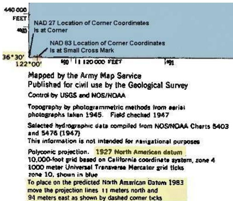
This is an example of a US Geological Survey topographic map that has been updated from NAD27 to NAD83 in this way. The basic map is the old NAD27 map. You must read the legend and make an adjustment if you want NAD83 (the same as WGS84) coordinates. The location of the corner coordinates is also show as a small cross in each corner. This is very useful in deciding whether to add or subtract the adjustments.
